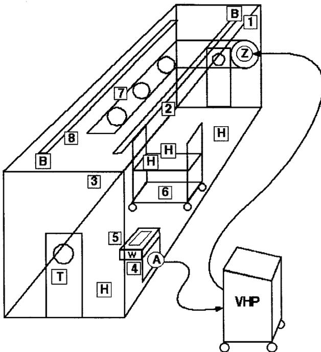
**Figure 1.** Animal room set-up for decontamination. (A) exhaust air; (B) light fixtures; (H) air fan heaters; (T) thermohydrograph; (VHP) VHP 1000 unit (outside room); (W) hand basin; (Z) air inlet; (1 through 8) locations of biological and chemical indicator strips.
